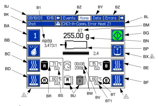
Temperature status will only be displayed if heaters are installed and enabled.
